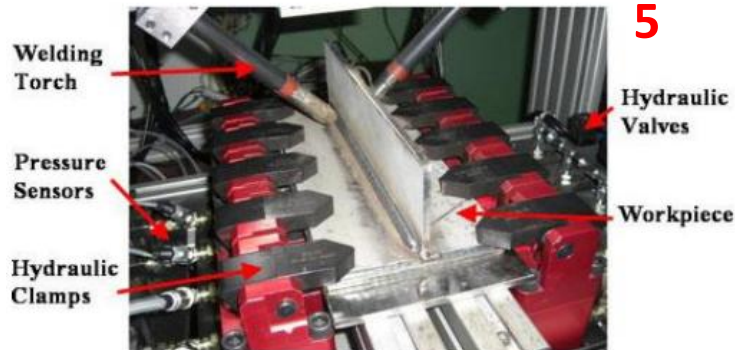
Schematic representation of static thermal tensioning process
