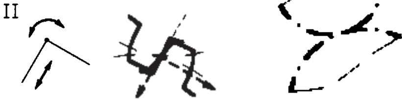
Fig. Number of degrees of freedom, schematic representation and symbolic representation of gear joint [Gronowicz 2003]
