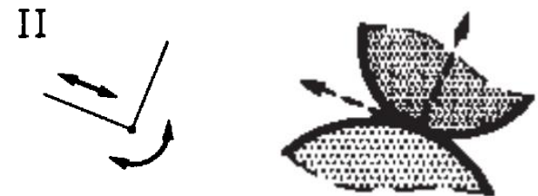
Fig. Number of degrees of freedom and schematic representation of cam and follower [Gronowicz 2003]
