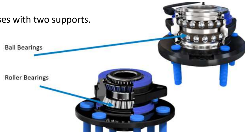
Fig. Single support arrangement: wheel bearing [https://www.mevotech.com/article/wheel-bearings-and-hubs-101-what-you-need-to-know/]
