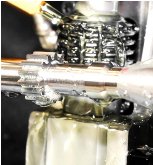
Fig. Hobbing spur gear [ https://en.wikipedia.org/wiki/Hobbing ]
