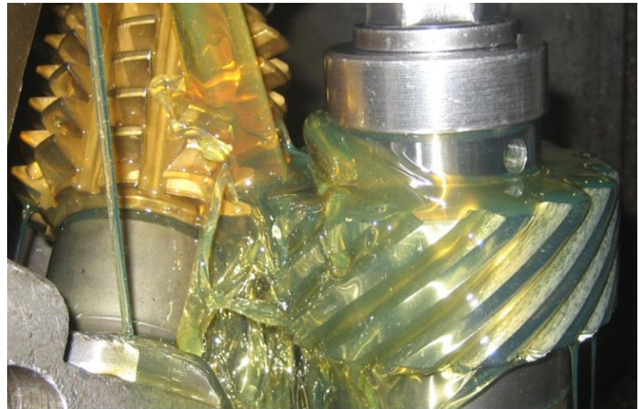
Fig. Hobbing helical gear [ http://vestavia.eu/product/manufacturing-helical-gears/ ]
