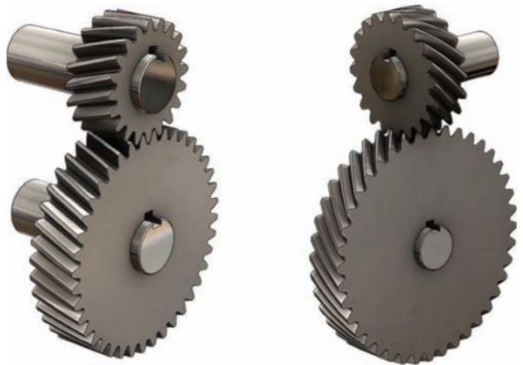
(a) Right hand and left hand helical gears with 20° helix angle and parallel axes
