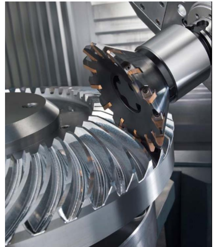
Fig. Milling proces by disc mill cutter – 5 axis CNC machine [ https://www.geartechnology.com/articles/0317/5-Axis_Gear_Manufacturing_Gets_Practical/ ]
