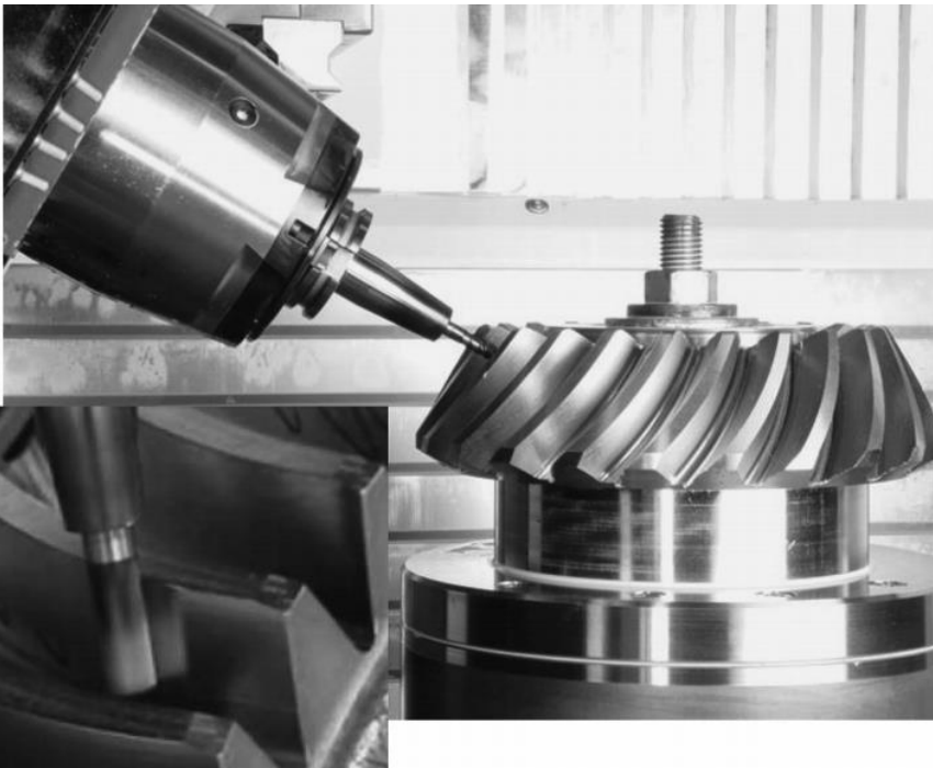
Fig. Milling proces by end mill cutter – 5 axis CNC machine [Radzevich 2017]
