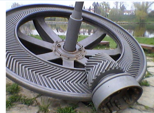
Fig. Herringbone bevel gears (made by Citroen) [ https://en.wikipedia.org/wiki/Herringbone_gear ]
