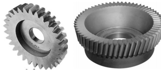
Fig. Gear shaper cutter - spur gears [Radzevich 2017]
