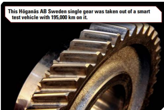
Fig. Powder metal gear [ https://www.geartechnology.com/articles/0917/What's_New_and_Noteworthy_in_Powder_Metal/ ]
