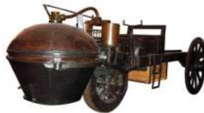
Nicolas-Joseph Cugnot - French inventor 1769 (small version) - First self-propelled mechanical land-vehicle, steam engine [ https://pl.wikipedia.org/wiki/Nicolas-Joseph_Cugnot ]
