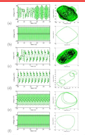
Figure 3: Voltage open circuit time series and the corresponding phase portrait with delayed coordinate (delay was fixed to one quarter of excitation period) for  $\alpha = 0.35, 0.78, 1.00, 1.195, 1.25$  for a-f, respectively.
