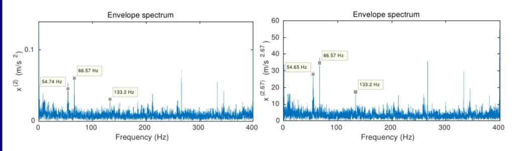
Figure 5. Envelope spectra of acceleration and  $x^{(2.67)}$  from the pump when cavitation occurs, band pass filtering from 1000 Hz to 2000 Hz
