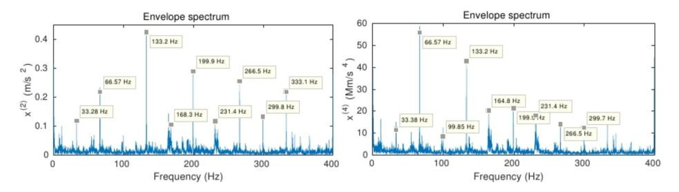
Figure 4. Envelope spectra of acceleration and snap from the gearbox when cavitation occurs, band pass filtering from 1000 Hz to 2000 Hz
