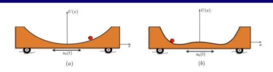
Fig. 5 The dynamics of a nonlinear energy harvester can be fairly well understood via a simple analogy with a particle moving along a cart. (a) Monostable potential and (b) bistable potential.
