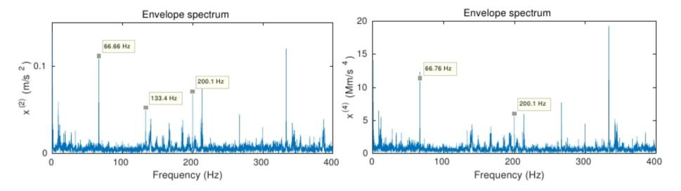
Figure 7. Envelope spectra of acceleration and snap from the pump without cavitation, band pass filtering from 1000 Hz to 2000 Hz
