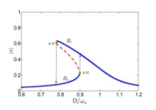
Fig. 10 Frequency response of the particle in a single potential well of the bistable potential system when  $A < A_1$ . Dashed lines represent unstable periodic responses.
