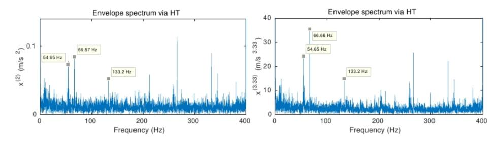
Figure 8. Envelope spectra of acceleration and  $x^{(3.33)}$  obtained via Hilbert transform from the pump when cavitation occurs, band pass filtering from 1000 Hz to 2000 Hz
