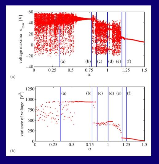
The fractional order of damping makes the significant changes in the system response. The system goes through several bifurcations with changing  $\alpha$ .
