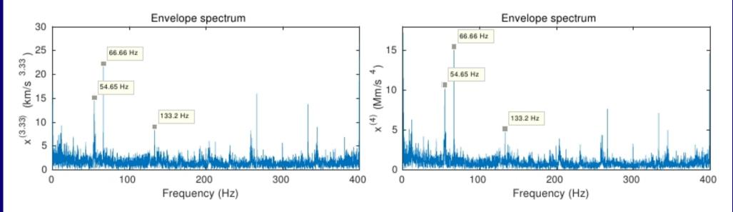
Figure 6. Envelope spectra of  $x^{(3.33)}$  and snap from the pump when cavitation occurs, band pass filtering from 1000 Hz to 2000 Hz
